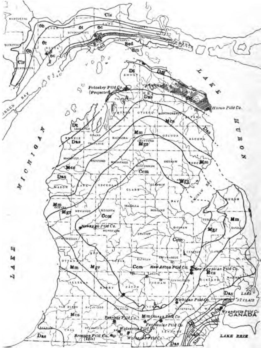
Figure 4. Geological map showing location of Portland cement plants and principle areas in which occur deposits of limestone and shale suitable for use in making Portland cement.
